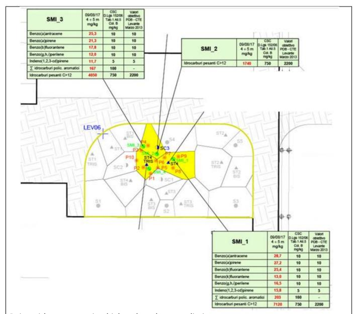
Point with concentration higher than the remediation target
