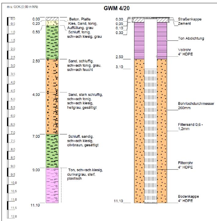
The results of pump testing conducted over 72 hours in the upper aquifer sediments determined an average hydraulic conductivity of  $1.3 \times 10^{-6}$  m/s indicating an aquifer of marginal yield (2L/min), due to the presence of significant silt and clay fines within the aquifer matrix. The direction of groundwater flow is to the south-southwest with a hydraulic gradient of approximately 5%.
