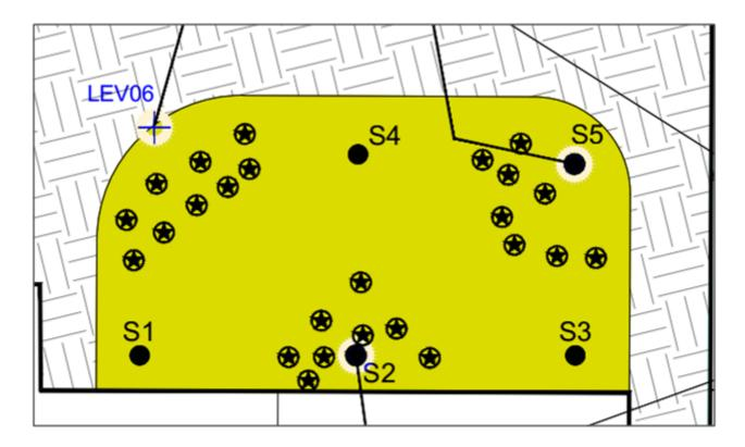
Following the injection of the oxidizing mixture, the remediation monitoring activity was carried out, which included the execution of n. 4 boreholes, with a fortnightly frequency, up to 5 m deep, for a total of 3 survey campaigns from 01/08/2016 to 29/08/2016 (T1, T2 and T3). In this way, the effect of the oxidizing mixture was monitored respect to the portion of soil subject to remediation (between 3.0 m and 5.0 m of depth from the
