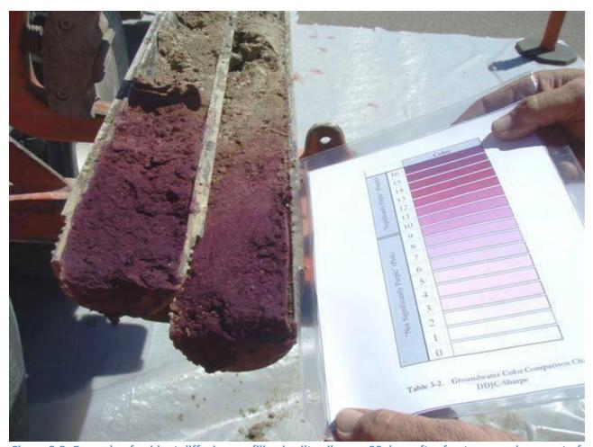
Figure 2.8- Example of oxidant diffusion profiling in silt soil cores 90 days after fracture-emplacement of potassium permanganate oxidant slurry (photo courtesy of URS, Bures archive)
