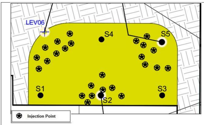
First cycle of treatment with sodium carbonate
