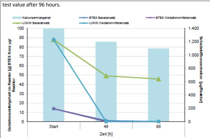
Oxidant consumption (KMnO<sub>4</sub>) and contaminant reduction (CHC and BTEX) during 96 hr reactor test
