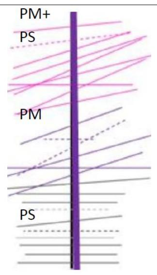
From 6 m bgs to 7.5 m bgs a mixture of solid permanganate and persulfate was injected. This was probably the first time when both agents were injected simultaneously. Thereafter, only solid permanganate was injected. The loading ranged from 150 to 250 kg per frac. From 9 m depth onwards only persulfate solution (50% concentration) was injected.
