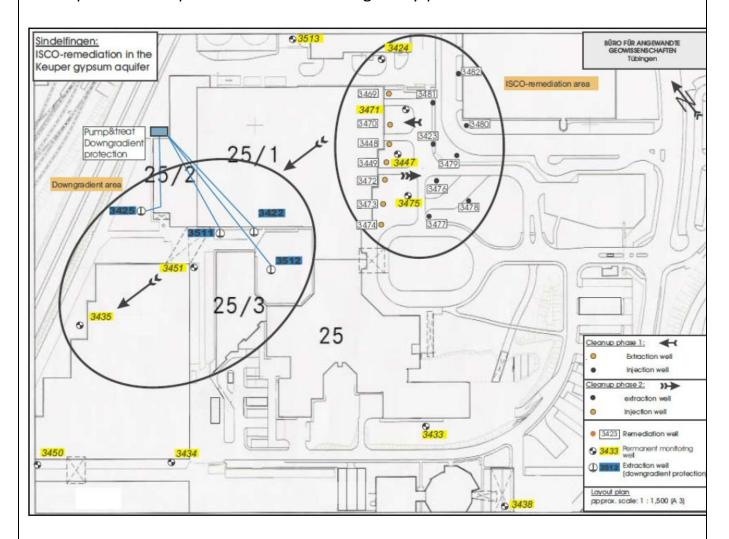
ISCO remediation of the Keuper gypsum aquifer. Layout plan with ISCO cleanup area and downgradient area
