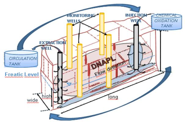
Figure 2.4- 3D Scheme recirculation system
