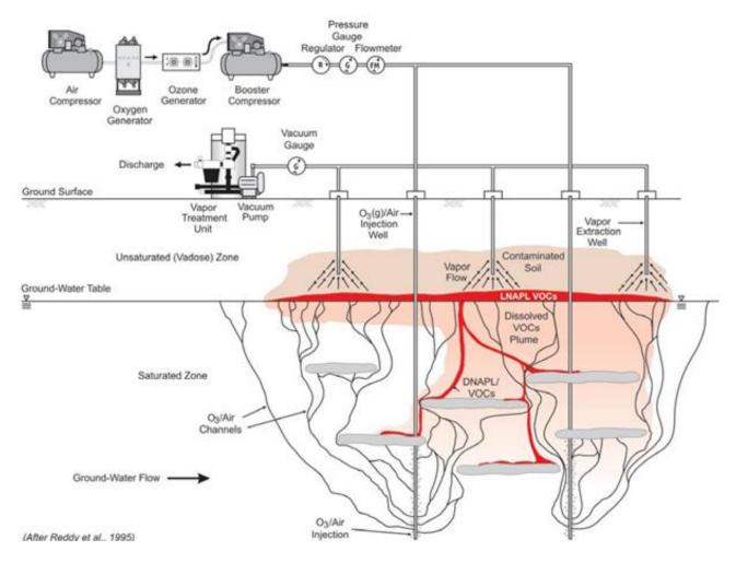
Figure 2.9- General conceptual model of in-situ ozonation in the saturated zone with soil vacuum extraction to capture volatile emissions and O<sub>3</sub>.
