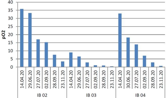
Typical oxygen depletion profile in plume area wells after injection
