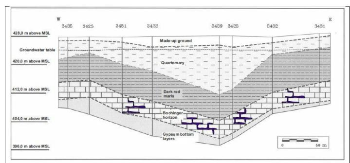
Geological cross-section in west-east direction, schematic
