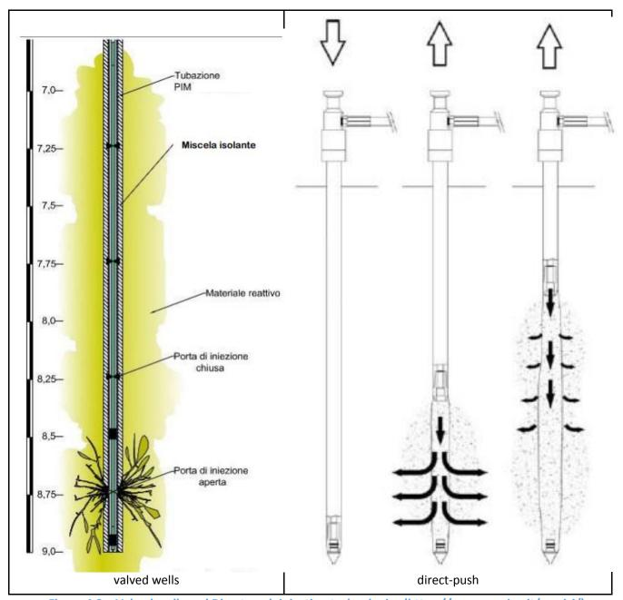
Figure 4.2 – Valved wells and Direct-push injection technologies (https://www.carsico.it/servizi/)
