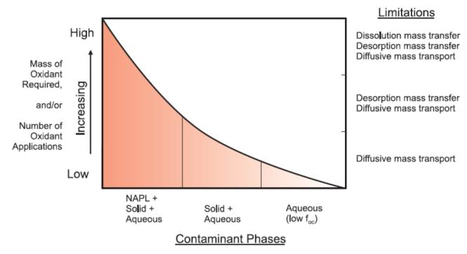
Figure 3.2- Impact of contaminant phases, mass transfer, and mass transport limitations on the mass of oxidant and/or the number of oxidant applications needed for ISCO
