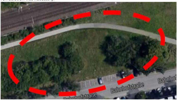
Because parts of the subsurface contamination are located below a main road (see picture below)with services including a sewer, gas pipeline, telecommunications only in-situ remediation technologies were deemed feasible for remediation of this specific sub area. A variety of methods were evaluated including thermal but from a cost-benefit viewpoint was ISCO using hydraulic fracturing as the preferred method.
