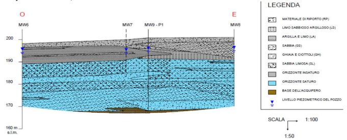
The local outflow of the aquifer is E-W in the portion of the site involved in the intervention. The average hydraulic gradient is equal to 0.5% and the permeability varies from  $4.4 \times 10^{-5}$  m/sec to  $5.5 \times 10^{-5}$  m/sec, the flow rate of the groundwater has been calculated equal to about 40 m/year.
