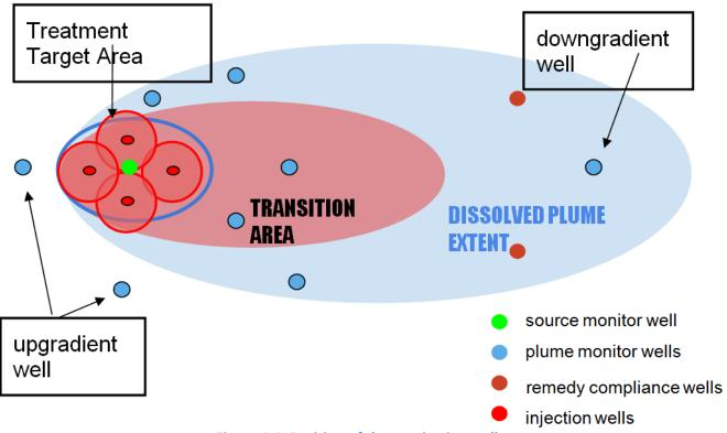
Figure 4.4: Position of the monitoring wells
