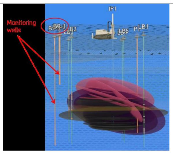
Furthermore, we were able to observe reagents in two groundwater monitoring wells screened in either the clayey silt layer and the weathered marlstone, which are located 7 m away from the injection bore aligned with the smaller axis of the ellipsoids (see picture left).
