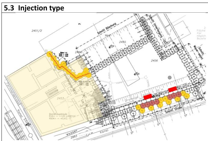
A plan view of the site. Bright red indicates sources of contamination (sewer, washing machines), red and yellow circles are planned HaloCrete columns. Column spacing was 1.2m to secure statical required overlapping, column diameter 1.5m. Drilling depths of up to 9m bgl
