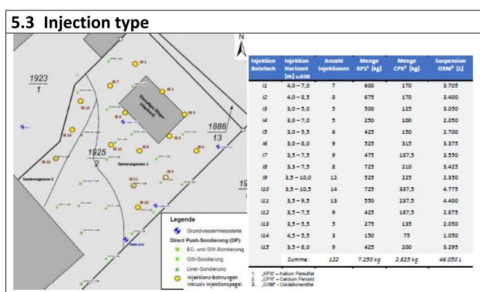
The fracture-emplacement of oxidant slurry using TSE® technology was achieved by advancing drill rods using Direct Push drilling equipment into subsoils to predetermined depths, followed by injection of slurry under hydraulic pressure using specialized high-pressure injection assemblies, and pumping and mixing equipment. The injections were conducted in a "top-down" approach, at 0,5 m depth intervals to the maximum depth of
