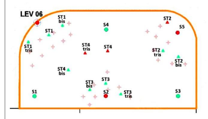
Samples to monitor remediation (ST, STbis, STtris), green means that the target concentration was reached, red means that the target concentration was not reached
