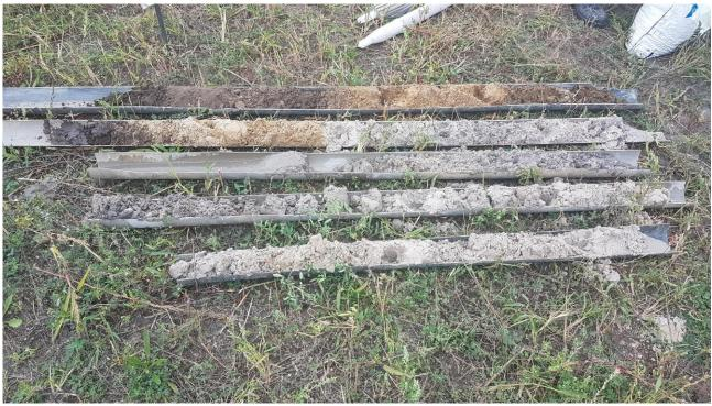
Drill core borehole (sonic drill)
