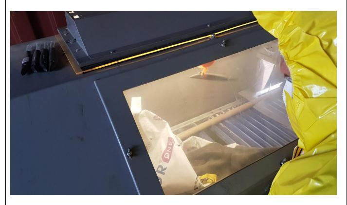
The injections were made per batch, and in the injection plan there are several different concentration batches provided. A typical batch contained 4 m<sup>3</sup> of clean water into which a specified amount of Klozur One was added. From the mixing unit, the proper solution of Klozur One is transferred into the injection tank.
