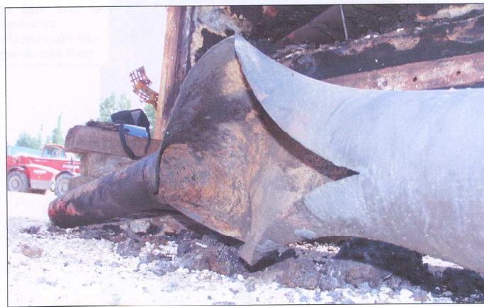
Views of the ruptured tube
