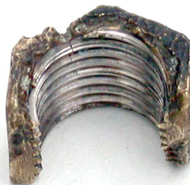
Fig. 8. Piece of the defective nut
