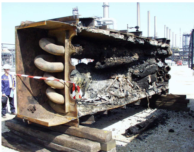
Partial view of furnace 42F201 after the fire and dismantling for inspection
