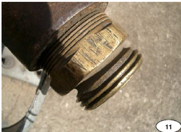
Examples of worn threaded coupling : road-tanker fitting and threaded ring
