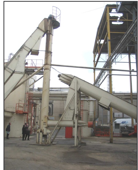
Mechanical transport with decoupling by screw
