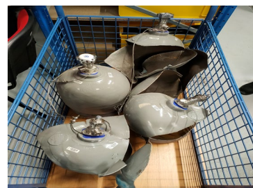
LP cylinders after the accident
