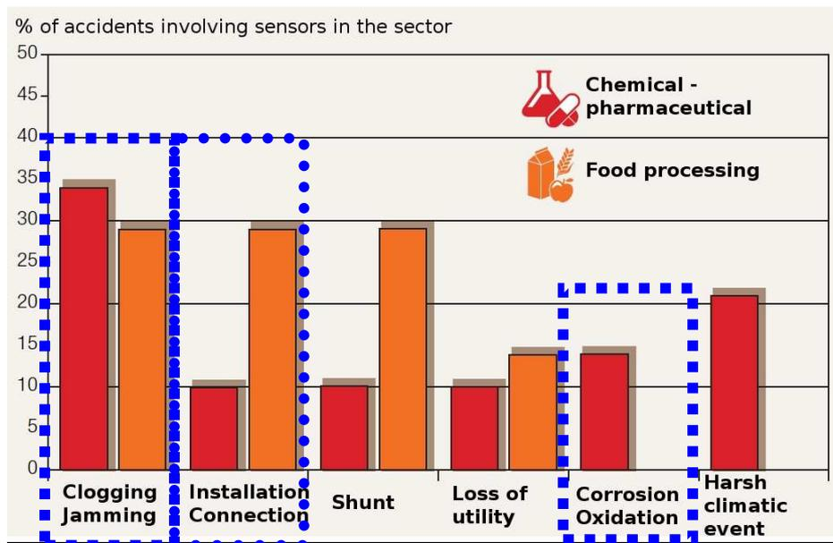
Fig. 5 : Primary causes of sensor malfunction for the chemical and food processing sector (ARIA base)
