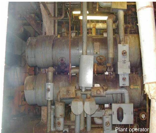
The accident occurred inside an isocyanate production workshop. The process implemented consisted of generating a reaction from a phosgene solution on an amine compound under conditions of high temperature and pressure.
