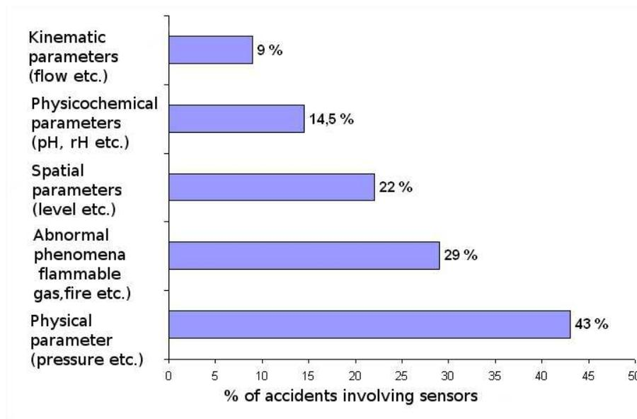
Fig. 3 : Breakdown of the functions performed by sensors involved in the analysed sample of accidents (ARIA base)
