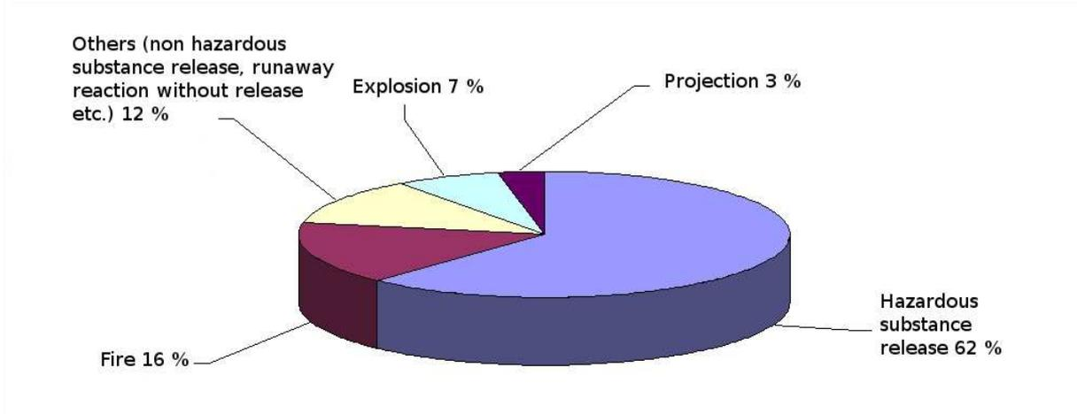
Fig. 2 : Breakdown of phenomena caused by accidents involving sensors (ARIA base)
