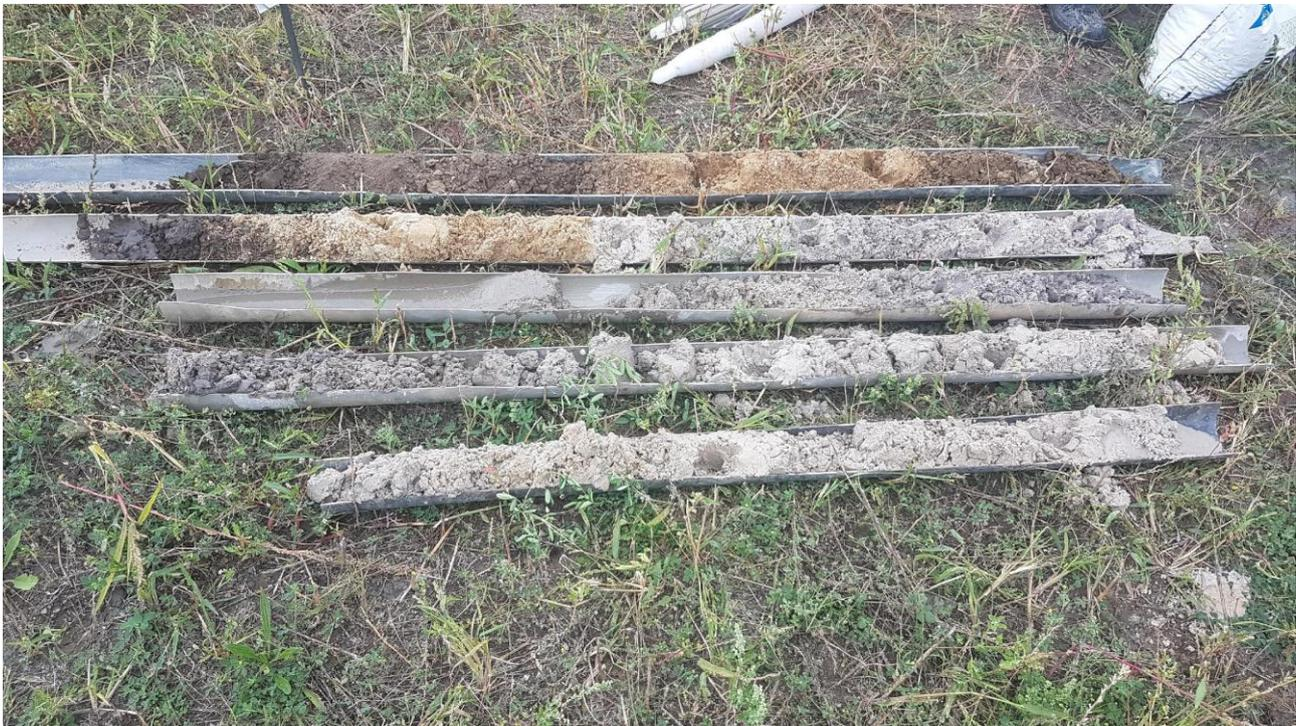
Drill core borehole (sonic drill)
