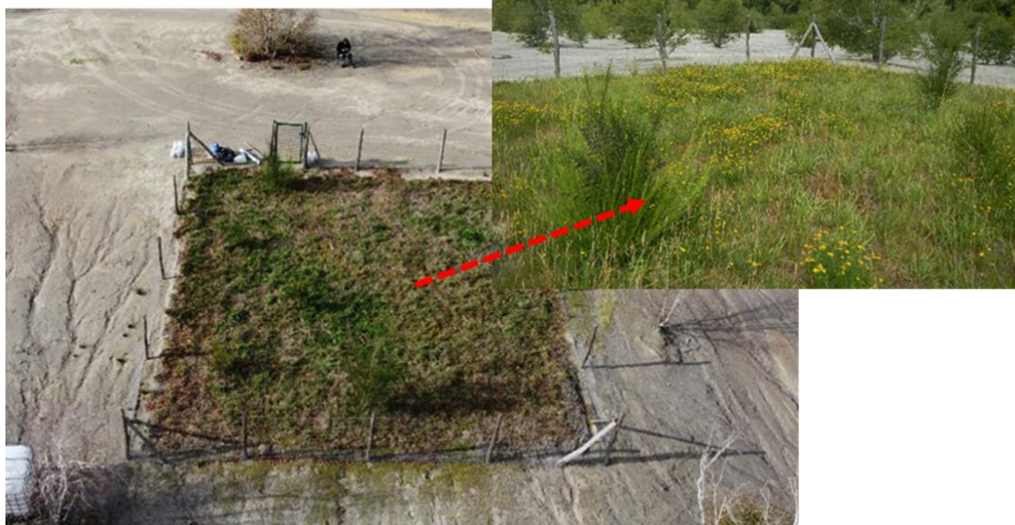
Figure 9 - Plot on the tailing slope (rather dry and intense erosion)
